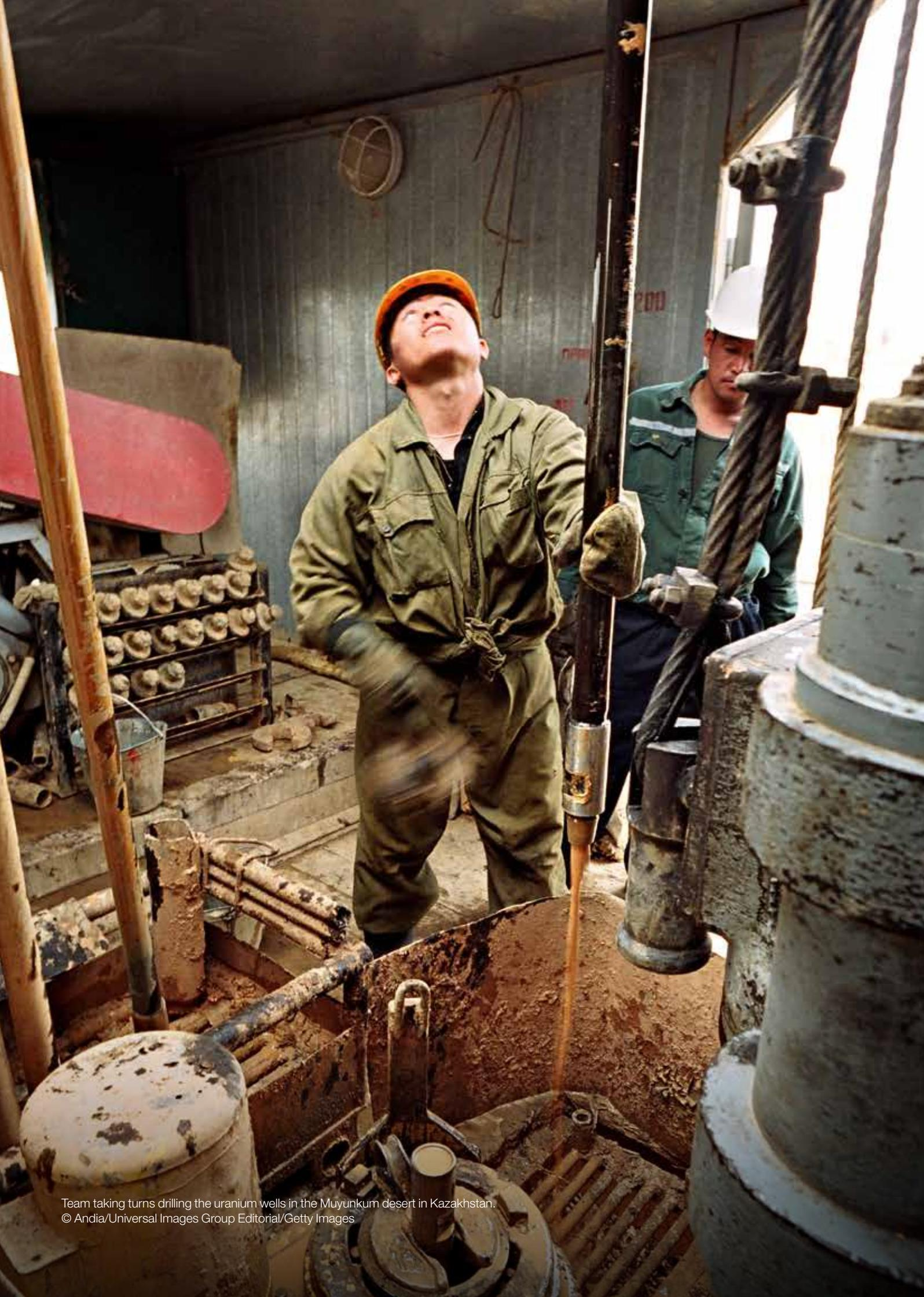
Team taking turns drilling the uranium wells in the Muyunkum desert in Kazakhstan.
